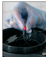
3. Insert the correct nozzle in the injector (see the nozzle directory on the following page).
